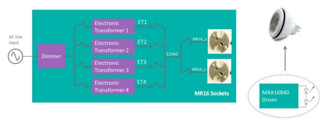
The demo includes a set of four electronic transformers which convert the line voltage to the 12V required by the MR16 bulb. A trailing edge dimmer precedes the electronic transformers and is used to turn the bulbs on and off and to dim the bulbs.
