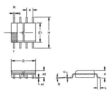
The chamfer on the body is optional. If it is not present, a terminal 1 identifier must be positioned so that ½ or more of its area is contained in the hatched zone.
