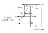
Measuring a 4-20mA loop current.
