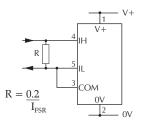
Measuring current. The meter's supply is isolated from the current being measured.
