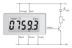
Using the PULSE O/P to drive an LED. The LED will illuminate once after every hour.
