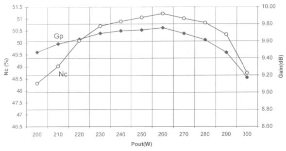
Collector Efficiency and Power Gain vs. Power Output Vcc=36VDC, Pulse Width=100µS, Duty=10%, 2.8GHz
