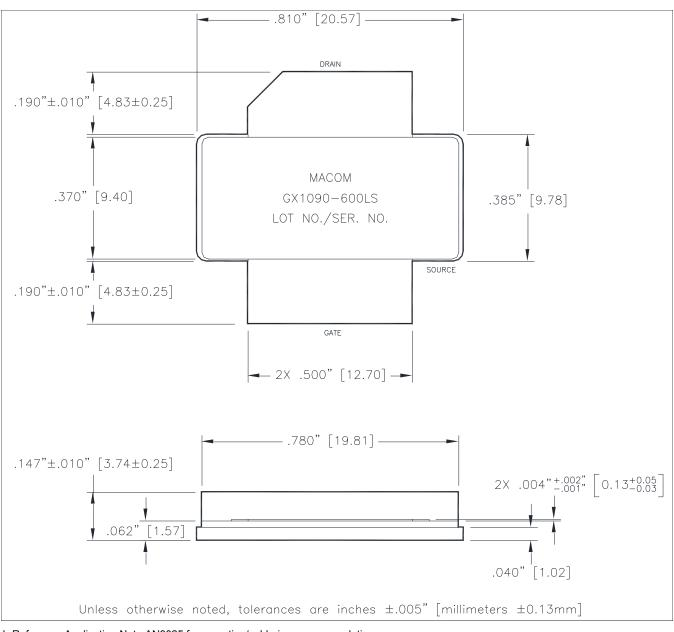
† Reference Application Note AN3025 for mounting/soldering recommendations. Meets JEDEC moisture sensitivity level 1 requirements. Plating is Ni/Au.
