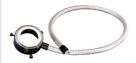
Fiber Optic Ring Light, with its continuous ring, is the most popular light transmitter. The ring light housing encases high-quality glass fibers to provide  $360^{\circ}$  shadow-free uniform illumination that makes viewing of inspection and assembly applications a snap. Its 36'' cable, made with interlocking stainless steel sheathing, enables the illuminator to be positioned outside the immediate work area to provide more space for inspection and assembly operations.
