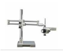
The Dual Boom Ball-Bearing Stand features a 26' stainless steel horizontal boom extension (limited to 24" when used with a System 373 model) and a 17.5" vertical boom mounted to a 10" x 10" die-cast base. Ball-bearing design allows fluid horizontal extension of the boom stand. The focus mount angles to 45° to permit additional viewing and inspection perspectives. For use with all Luxo System 273, 373 and VIP microscopes.
