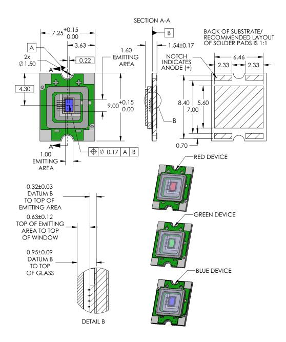
• Red, Green and Blue SBT16 PhlatLight  $^{TM}$  LEDs are individually assembled into a SMT Board with a footprint of 9.0 mm x 7.25 mm.
