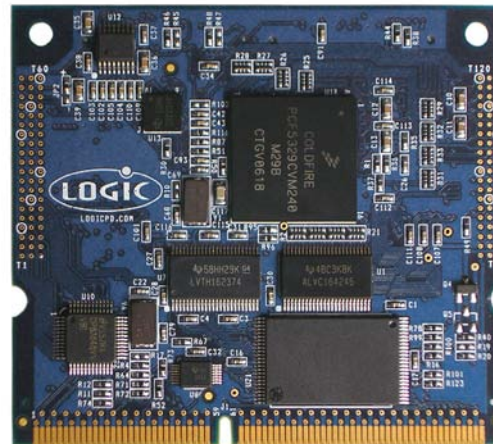
FREESCALE MCF5329 FIRE ENGINE
