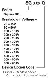
Blank) = Standard device **Q** = Quick Response Version (300V, 350V, 420V, 450V, 500V, 600V only)
