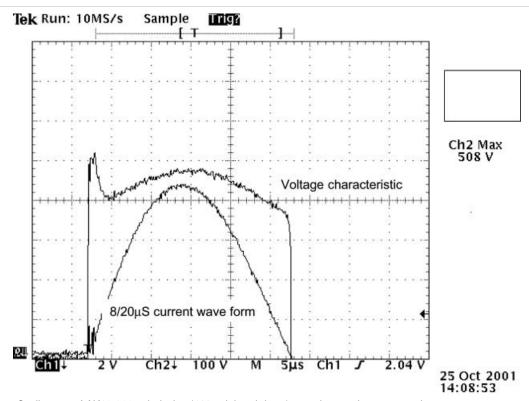
Oscilogram of AK10-380 volt device (422 volt breakdown) tested at maximum surge duty using 10,000 Amp 8/20µS wave form: maximum clamping voltage is 508 volts.
