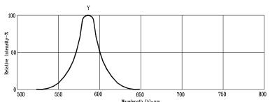
$\label{eq:wavelength} \begin{tabular}{ll} Wavelength $(\lambda)$-nm. \\ Fig1. RELATIVE INTENSITY VS. WAVELENGTH \\ \end{tabular}$
