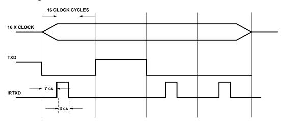
The encoder sends a pulse for every space or "0" that is sent on the TXD line. On a high to low transition of the TXD line, the generation of the pulse is delayed for 7 clock cycles of the 16XCLK before the pulse is set high for 3 clock cycles (or 3/16th of a bit time) and then subsequently pulled low.
