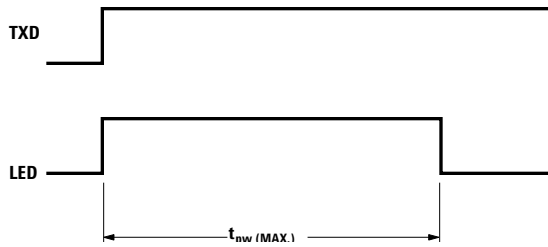
Figure 4. TXD "stuck on" protection waveform.
