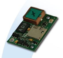
Laird Technologies' WISMC01 Wireless LAN Processor Modules are the world's most compact, feature-rich solutions for designers needing to add wireless connectivity to their products. With fully integrated drivers and stacks, this complete stand-alone, pre-qualified wireless solution requires minimum development to implement connectivity to any embedded product.
