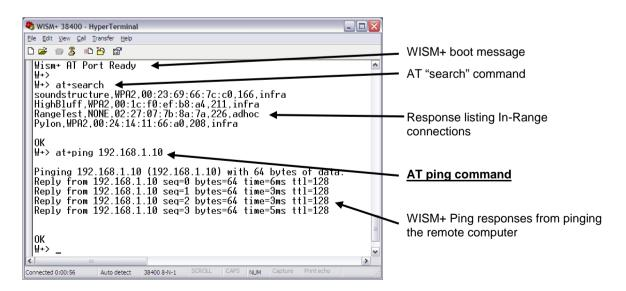
NOTE: In the ping command (shown above), the target of the 'PING' is the IP address of the remote PC configured in Ad-Hoc mode.
