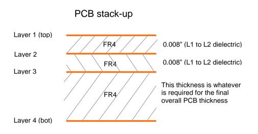
The Ethernet PHI interface requires good PCB design practices in order to yield acceptable EMI suppression. Use of ground plane which encloses noisy signals and clocks is imperative in order to produce a quiet design.
