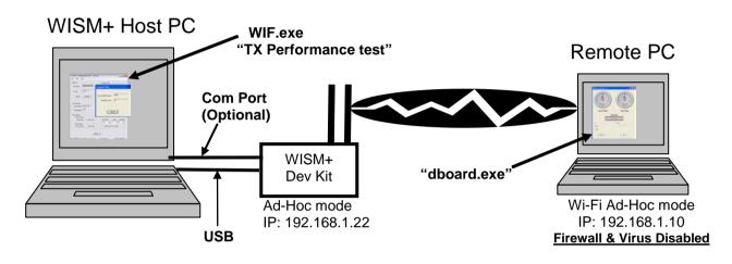
To begin, set up the Ad-Hoc connection between the WISM+ and the remote PC by following the procedure outlined in section: "Perform a Wireless Ping PC→WISM+".
