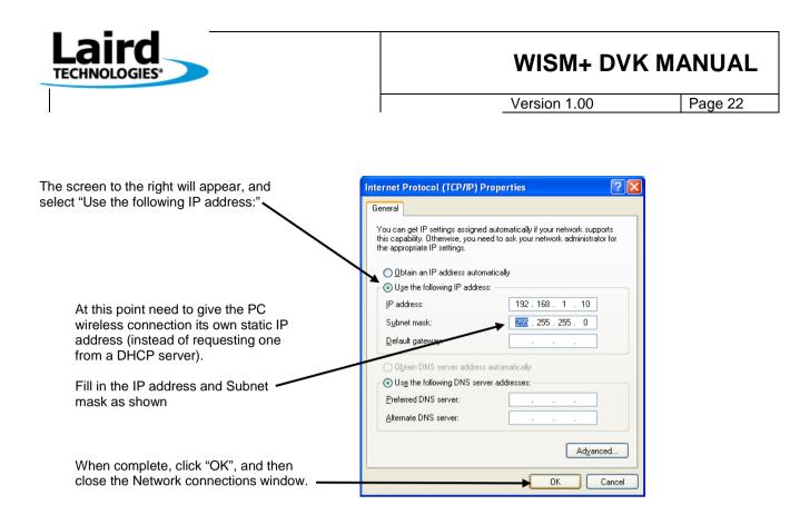
Now that we have given our wireless connection a static IP address, we are ready to allow the PC and WISM+ to join the Ad-Hoc connection.
