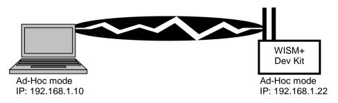
Since the WISM+ has been configured and reset into Ad-Hoc mode, now we have to go to the PC side and configure its Ad-Hoc wireless connection.
