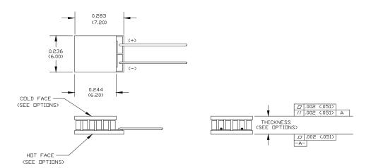
Solder Construction: 138°C, Bismuth Tin Tlam Substrates
