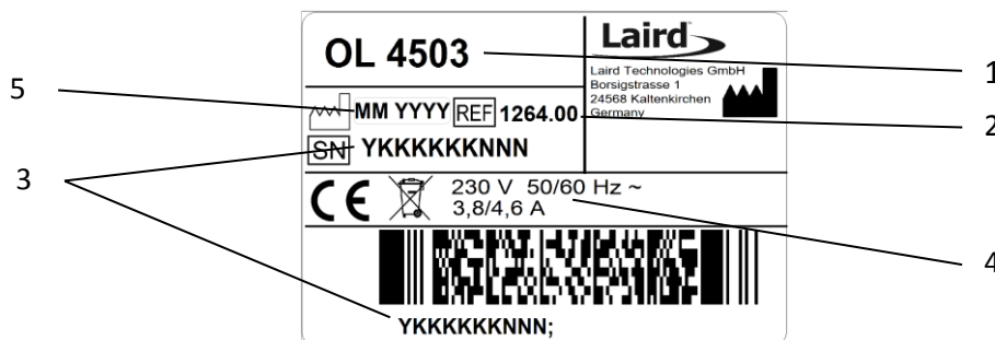
Fig. 2: Unit specific identification plate
