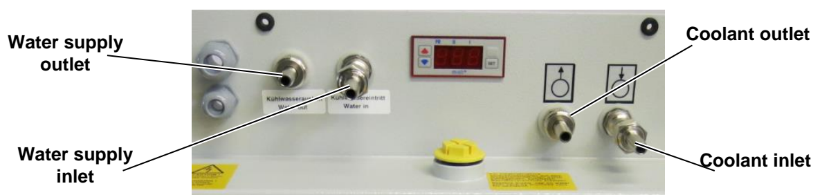
Fig. 8: Labelling of water inlet and water outlet
