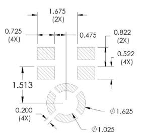
Notes: Dimensions are in millimeters unless otherwise specified. Detailed information on AP size considerations can be found in the latest *SiSonic<sup>™</sup> Design Guide* application note. Further optimizations based on application should be performed.
