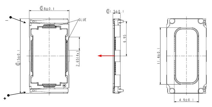
Positive voltage on pin '+' moves membrane in direction of red arrow!
