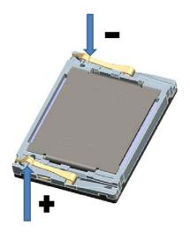
positive voltage on pin + moves membrane in direction of arrow
