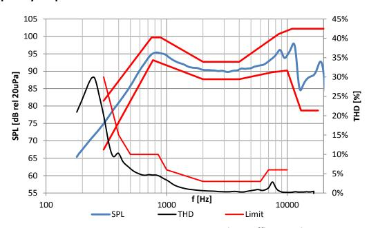
TYPICAL FREQUENCY RESPONSE measured on Baffle according to Chapter 2.4: distance d = 10cm, P= 600mW, 1ccm back cavity
