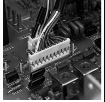
This 2.5mm (.098") pitch connector for printed circuit boards has an ultra-thin construction. The in-line method provides high-density capability to the end user.
