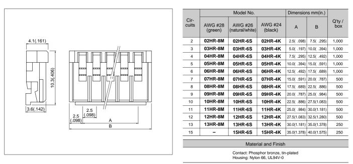
Note: 15HR-6S and 15HR-4K are not UL recognized nor CSA certified.
