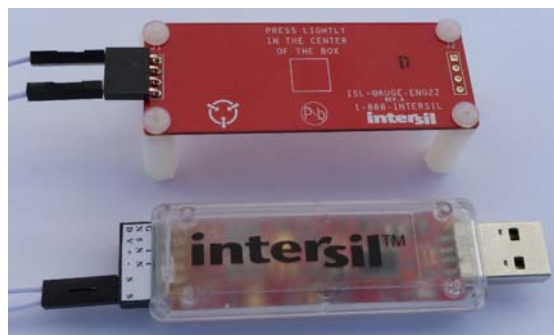
FIGURE 1. DAQ ON A STICK WITH STRAIN GAUGE
