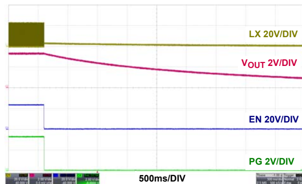
FIGURE 35. SHUTDOWN AT NO LOAD, PWM
