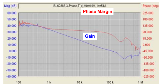
FIGURE 57. REFERENCE DESIGN LOOP GAIN T2(s) MEASUREMENT RESULT
