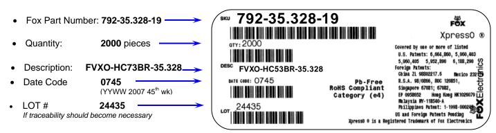
An additional identification code is contained internally if tracking should ever be necessary
