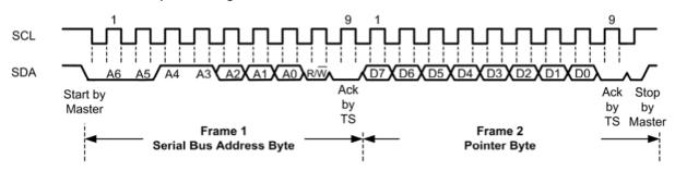
SMBus/I<sup>2</sup>C write to the pointer register followed by a write data word
