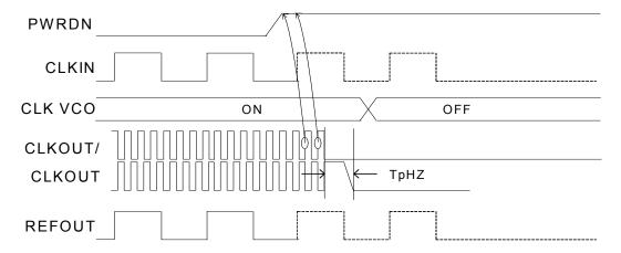
CLKOUT is driven differentially when PWRDWN# is de-asserted unless the CLKOUT is disabled through the SMBus register bit.
