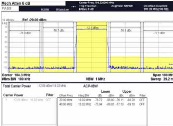
Fig 19. ACLR of 1 carrier LTE (BW=20 MHz) centered at 184.32 MHz
