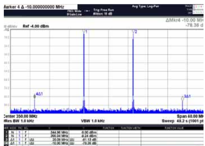
Fig 12. IMD3 (dBc) for two tones (spacing 10 MHz) centered at 350 MHz
