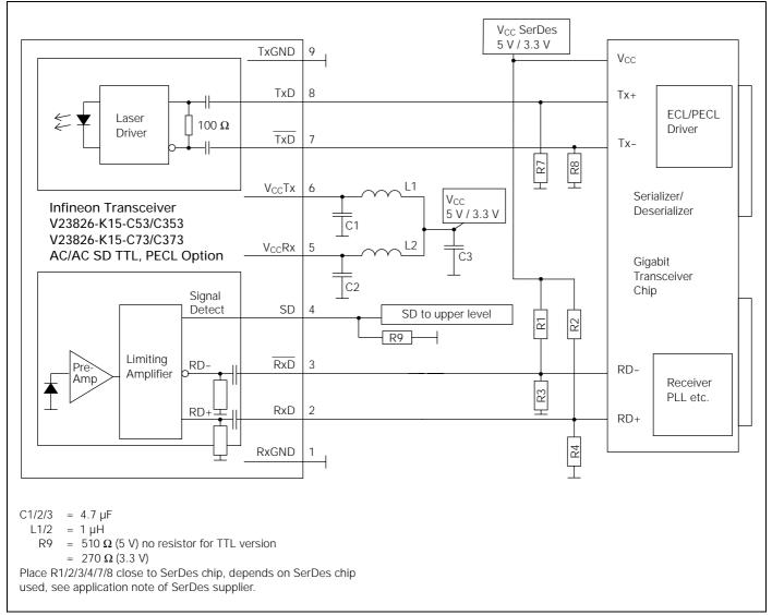
The power supply filtering is required for good EMI performance. Use short tracks from the inductor L1/L2 to the module  $V_{CC}Rx/V_{CC}Tx$ . We recommend a GND plane under the module for getting good EMI performance.
