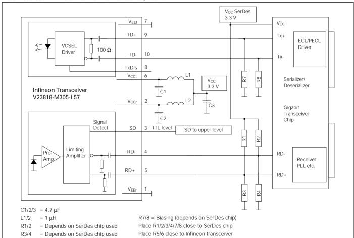
Values of R1/2/3/4 may vary as long as proper 50  $\Omega$  termination to  $V_{EE}$  or 100  $\Omega$  differential is provided. The power supply filtering is required for good EMI performance. Use short tracks from the inductor L1/L2 to the module  $V_{CC}Rx/V_{CC}Tx$ .
