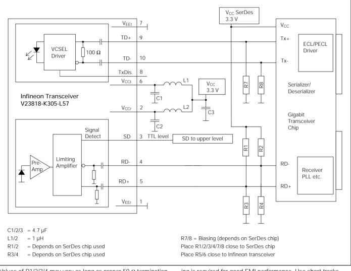
Values of R1/2/3/4 may vary as long as proper 50  $\Omega$  termination to V\_EE or 100  $\Omega$  differential is provided. The power supply filter-
