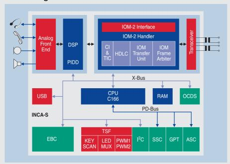
The typical application for the INCA-S is terminal equipment in which microphone, loudspeaker, headset, and handset are directly connected to the Analog Front End.
