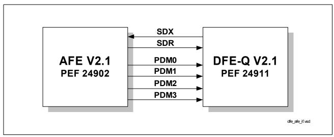
Figure 14 Interface to the Analog Front End
