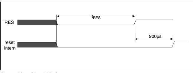
Figure 44 Reset Timing
