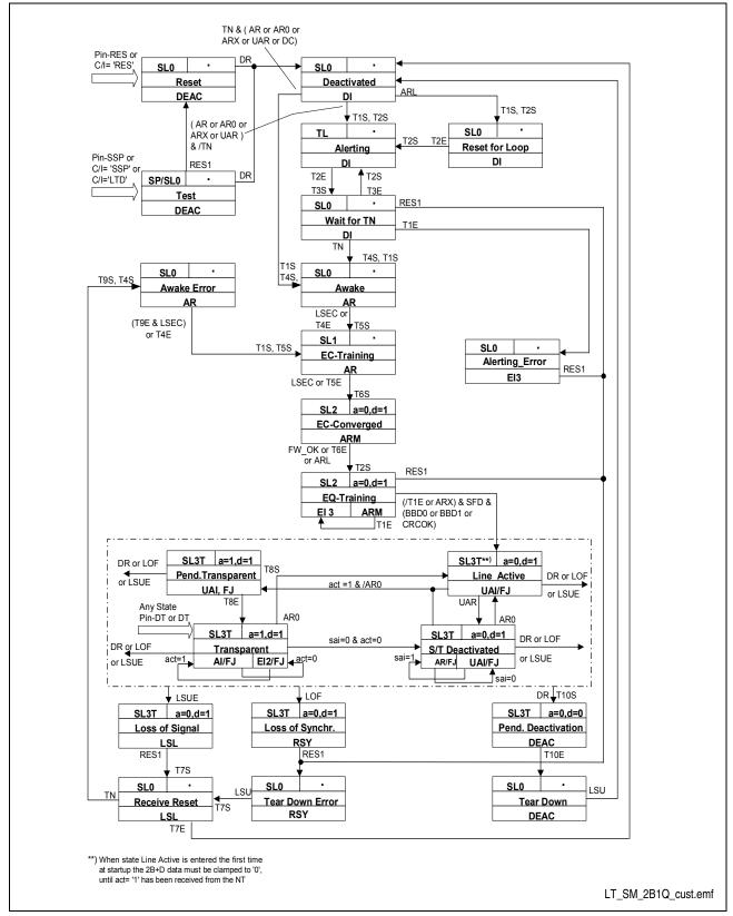
Figure 27 State Transition Diagram in LT-Mode
