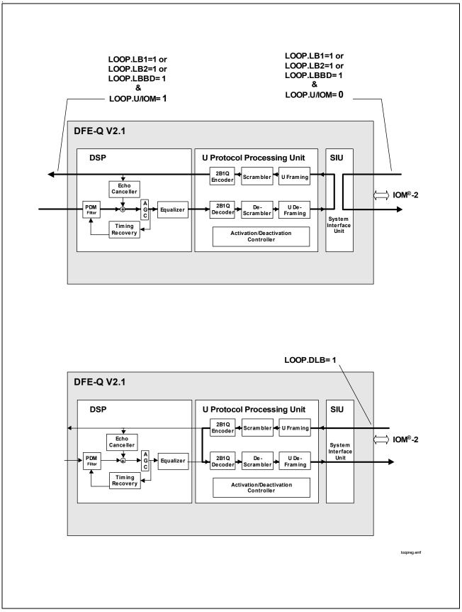
Figure 39 Loopbacks Featured by Register LOOP
