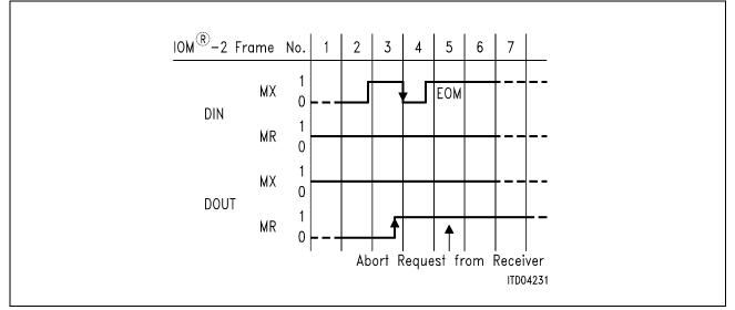
Figure 13 Abortion of Monitor Channel Transmission
