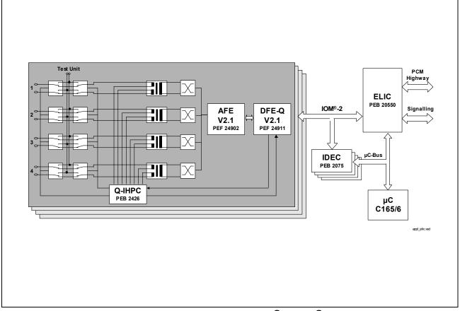
Figure 4 16-Line Card Application with ELIC<sup>®</sup>/ IDEC<sup>®</sup> Solution
