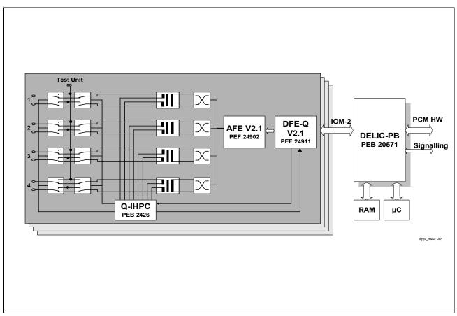
Figure 3 16-Line Card Application with DELIC Solution
