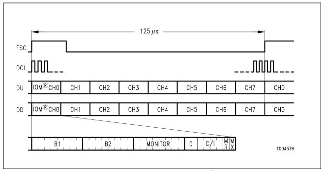
Figure 10 Multiplexed Frame Structure of the IOM<sup>®</sup>-2 Interface
