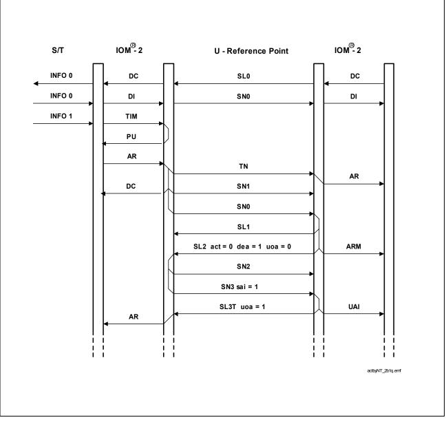
Figure 30 Complete Activation Initiated by TE
