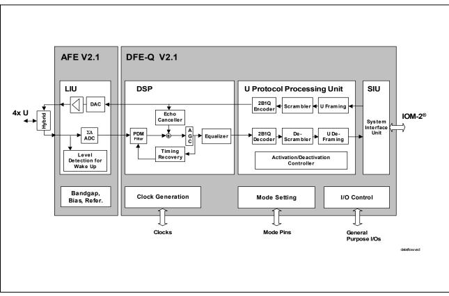
Figure 8 Block Diagram and Data Flow (DFE-Q V2.1 + AFE V2.1)
