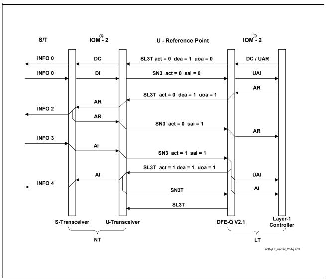
Figure 33 LT Initiated Activation with U-Interface Active
