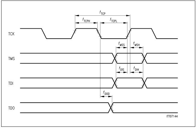
Figure 46 Boundary Scan Timing
