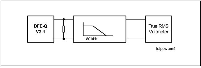
Figure 41 Total Power Measurement Set-Up
