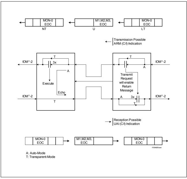
Figure 23 EOC-Procedure in Auto- and Transparent Mode
