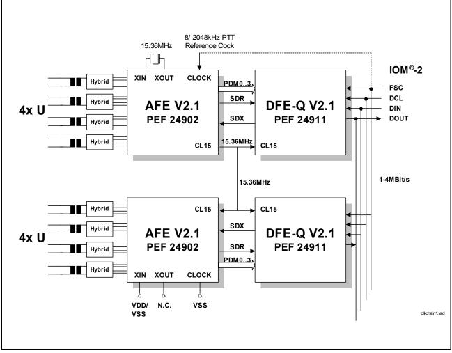
Figure 5 Connecting Two AFE/DFE-Q Chip Sets
