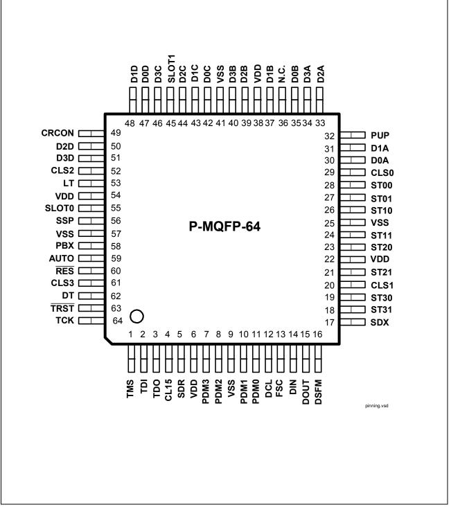
Figure 7 Pin Configuration (63 of 64 used)
