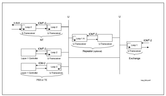
Figure 37 Test Loopbacks
