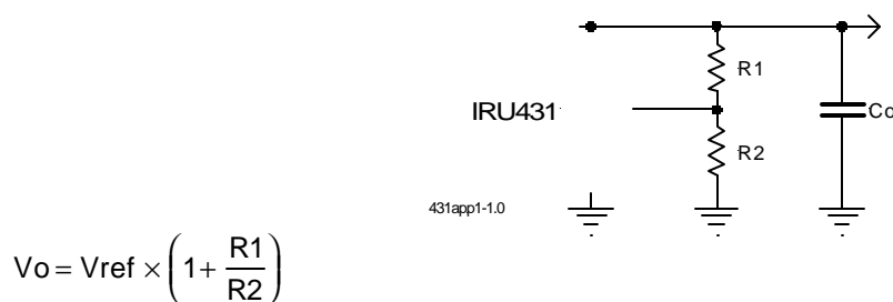
Typical application of the IRU431L as a shunt regulator / voltage reference
