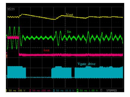
11.3.5 AC line jump test from 85VAC to 265VAC at full load
