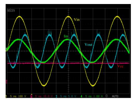
11.3.3 Load jump test at 230VAC, lout from 0.033A to 0.4A
