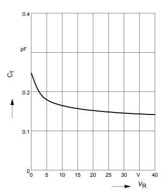
Line capacitance  $C_T = f$  (f)  $V_R = 0 V$
