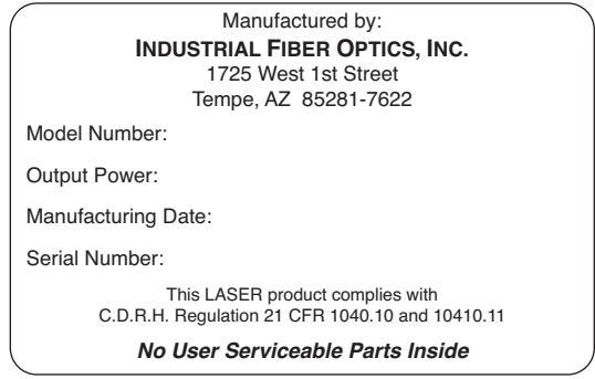
Figure 3. Laser certification and identification label.
