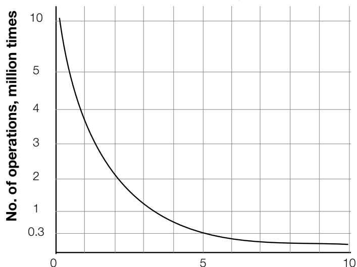
Life curve, resistive load (AC 240VC \cos \phi = 1 )
