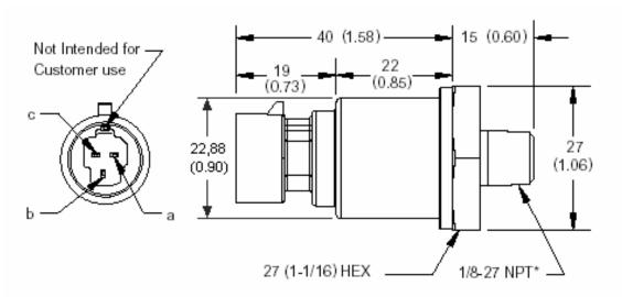
\* 1/4-18 NPT and G1/4-19 BSP configurations are both optional. Contact Honeywell to discuss other pressure port options.
