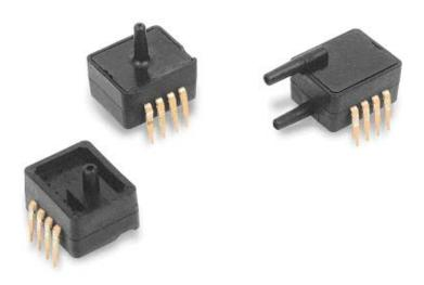
The ASDX series is an amplified version of Honeywell's proven performer and industry leading SDX series sensor. The amplified ASDX sensor's footprint is slightly larger than the SDX but it offers a high level output (4.0 Vdc span) on a very cost-effective basis. This series is fully calibrated and temperature compensated with on-board Application Specific Integrated Circuitry (ASIC). They are intended for use with non-corrosive, non-ionic working fluids; such as air and dry gases.
