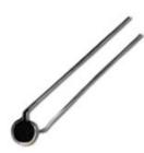
143 Series, 5,08 mm [0.2 in] disc thermistor with leads, 3,000 Ohm resistance, ±10.0% tolerance, 25/85 BETA = 3974
