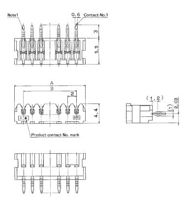
Note 1. The plug, which has the mark at the designated position, is for AWG26. Note 2. The cleaning by heat and trichloroethylene can't be implemented.
