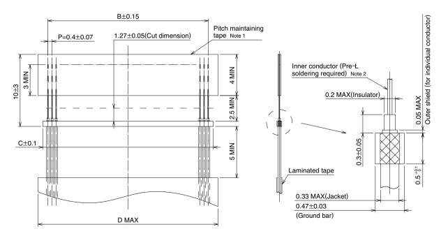
Note 1: The pitch maintaining tape can be left in place during the termination process. Use high quality tape.
