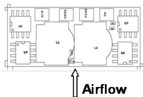
Figure 34. Airflow direction for thermal testing.
