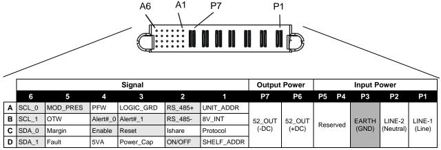
Connector is viewed from the rear positioned inside the power supply.
