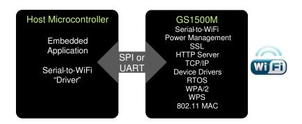
The GS1500M EVK Mrk II Evaluation Kit enables GainSpan customers to develop software on their existing microcontrollers to support the "AT" command set, and connect it to either UART or SPI interface on the evaluation kit reference board.
