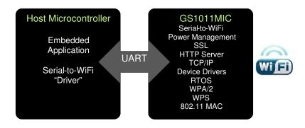
The GS1011 EVK Mrk IIc Evaluation Kit enables GainSpan customers to develop software on their existing microcontrollers to support the "AT" command set, and connect it through the UART interface on the evaluation kit reference board.
