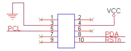
The ICP function uses only five pins: VCC, GND, PCL, PDA, and RSTn.
